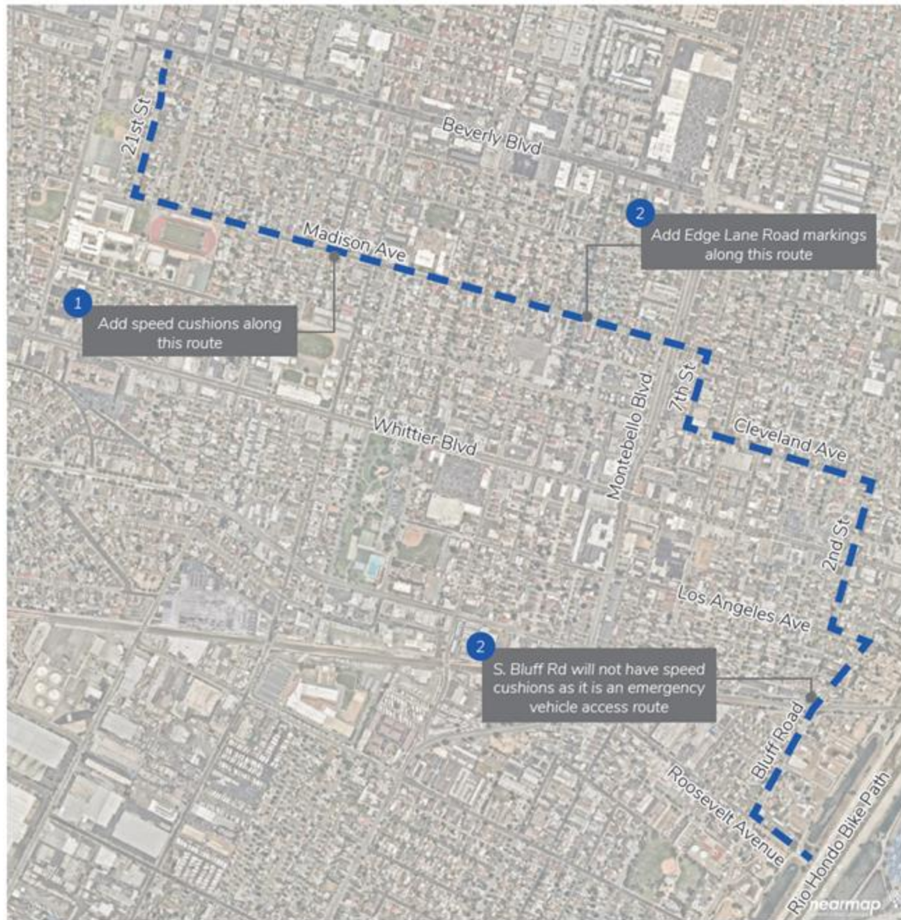
FIGURE 4-6: Neighborway with Edge Lane Road Markings and Speed Cushions
